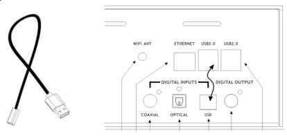
To ensure optimal Wireless performances, screw the provided wireless Antenna.
