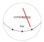
There is a bias indicator of power tubes V1~V8 set on the front side of transformers cover. Note: Normal operating point has been factory set at 50mA, the right point of the indicator. Don't leave the operating point beyond that point, the further right in this case.
