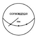
There is a bias indicator of power tubes V1~V8 set on the front side of transformers cover. Note: Normal operating point has been factory set at 55mA, the left point of the indicator. Don't leave the operating point beyond that point, the further right in this case.
