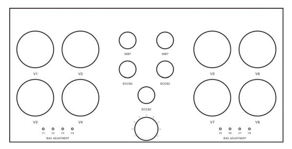
On the top cover lid: The holes of V1~V8 are bias adjustment. In the middle front there is a bias select switch/knob, which can select and indicate the bias of V1~V8 power tubes.
