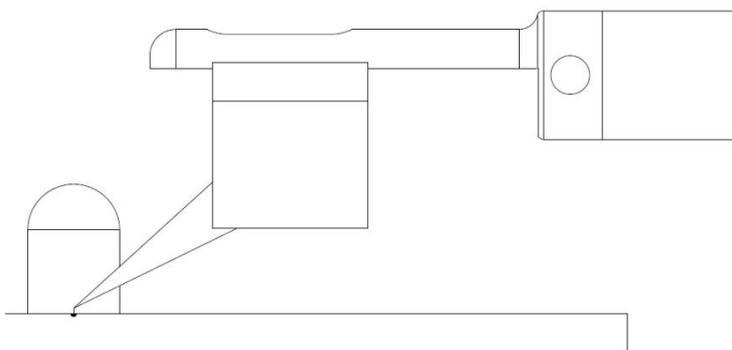
**Note1: It is very important to adjust the level of the air float tonearm. First you can adjust feet. If necessary, you also adjust the screw 1 confirm with the spirit level. In the end fix screw 2, 3 and 4.**
