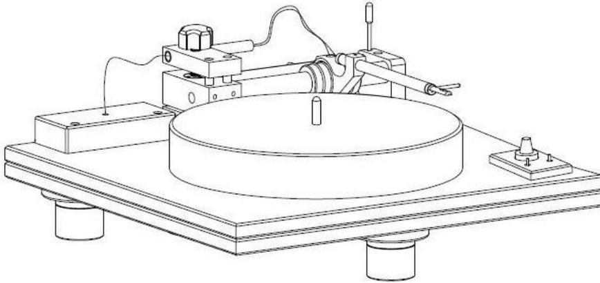
4. Remove the pump from the package. Follow the picture, make sure it use the air tube to connect with the water separator and tonearm. Then turn on pump. If the installation is correct, barometer will show 0.05MPa. Make sure the air bearing move is very smooth.
