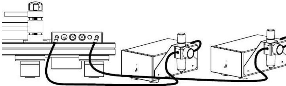
5. From left to right is: 33/45 speed selection switch, speed adjustment knob, power on/off switch. Put the Strobe Disc on the platter, and adjust the speed controller knob to get the 33.3rpm or 45rpm. The corresponding circle on Strobe Disc will display stable stripes.
