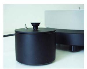
7. Take out one of the drive 'belts' and run it round the motor spindle and then round the platter. There are two ruts on the pulley of motor. The above rut is for 45 rpm, and the nether rut is for 33.3 rpm. Different ruts for the different speed. Only one switch control the motor. It could be found on the top of the motor housing and is a simple on/off.
