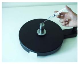
6. Put on the cotton gloves and pick up the acrylic platter, with the dip for the record label uppermost. Hold it level over the bearing housing, locate it carefully and gently lower it until it seats fully over the bearing.
