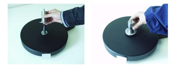
5. If it's not smooth enough, use the syringe to fill the small hole at the top of the spindle. Once you've done this turn the bearing whilst gently lifting the bearing housing. The oil will disappear into the bearing and wash down the shaft. Because of the very tight clearances of the bearing there may still be small amounts of 'friction' - this will disappear as the bearing runs in.
