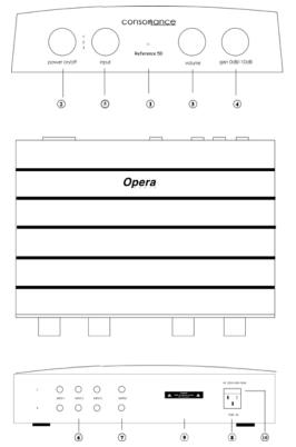
CONTROL FUNCTIONS: Volume left / right, Input Select, Power On/Off HARMONIC DISTORMS (for 2V RMS at output): 0.05%(70Hz-7kHz 4:1) FREQUENCY RESPONSE: (at -1dB) 3Hz-150kHz
