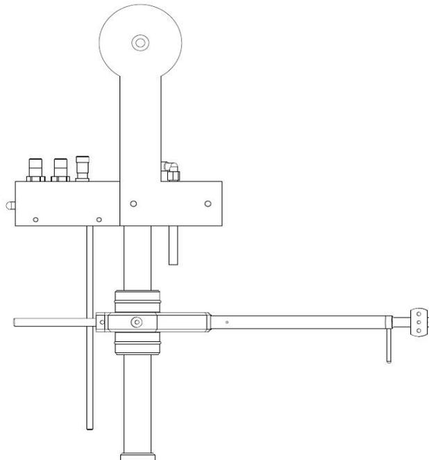
3. Use M6x35 screw to fix the tonearm on the turntable.
