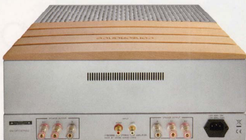
ABOVE: Just one set of single-ended RCA input sockets is provided, along with speaker terminals offering 4 and 8ohm taps from the amplifier's output transformer
